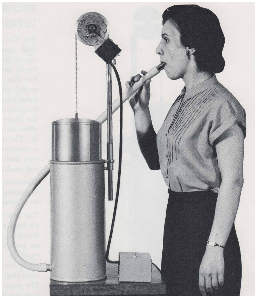
Timed Vitalometer, from W. E. Collins Inc., "A Catalog of Pulmonary Function Equipment and Accessories," 1966. The spirometer: a machine that measures human vitality through breath. Like all magical devices, it is both a product and projection of a cultural imaginary of the human body; its truth serves to reproduce an evolutionary understanding that biological differences naturally predispose the human to a social order whose differences are rendered environmental, thus, in turn, acting on breath itself.
